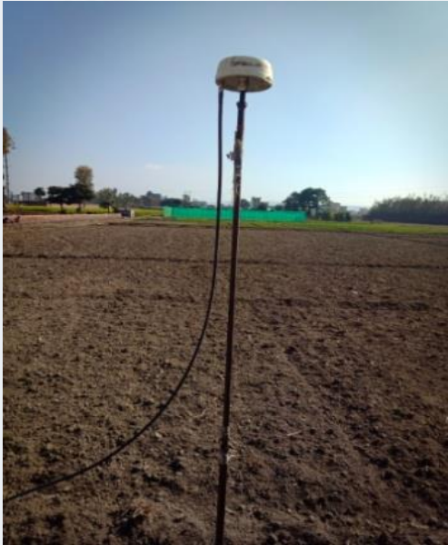
Field Photographs of NavIC Receiver deployment
