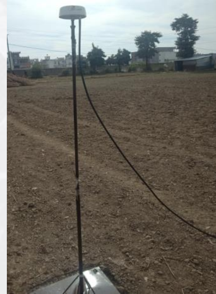
Field Photographs of NavIC Receiver deployment
