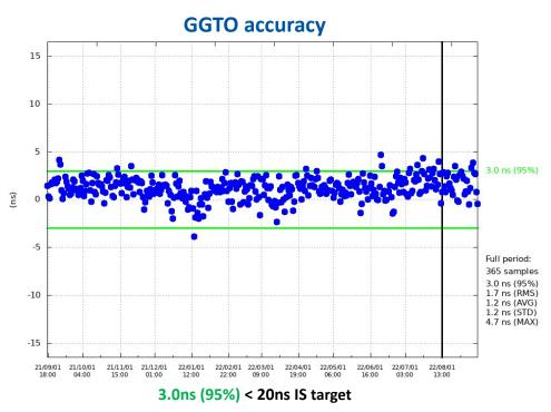
• Evaluated with calibrated timing GPS/Galileo receiver operated in UTC(k) laboratory (PTB, INRIM)
