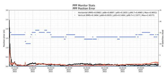
Initial HAS Galileo+GPS, 2f iono-free, float, open sky, static. Based on MagicPPP/PAULA project
