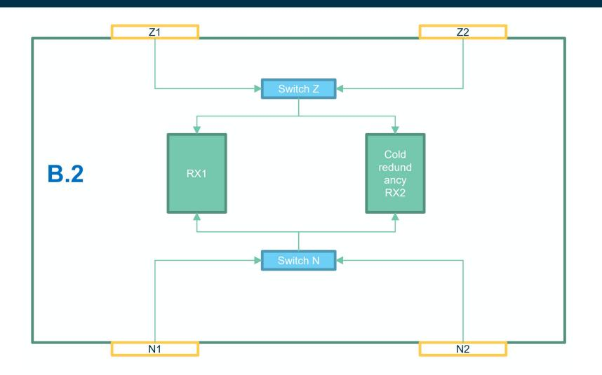
With redundant GNSS Zenit and NADIR antennas
