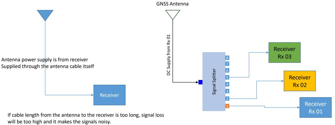
Check cable loss value for the cable
