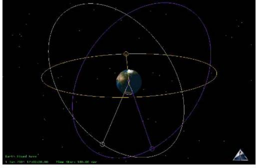
$(a=42, 164 \text{km}, e=0.099, i=45 \text{deg}, \Omega = 120 \text{deg apart})$
