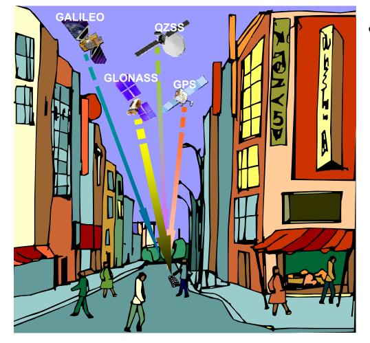
Ideal interoperability allows navigation with one signal each from four different systems with no additional receiver cost or complexity
