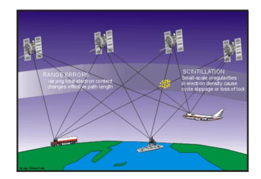
The ionosphere is defined as the region of the upper atmosphere where radio signal propagation is affected by charged particles.
