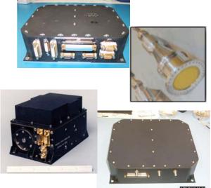
GPS, Signal and Instrument Processing Units, K/Ka-band horn, ultra-stable oscillator -- GRACE flight hardware provided by JPL
