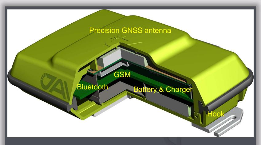
32 channels of GPS and GLONASS L1, code and carrier
