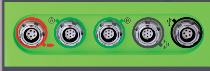
POWER SERIAL-A SERIAL-B ETHERNET USB
