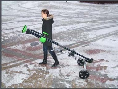
To make handling of the three additional antennas easy we have designed the RTK Umbrella. The receiver is mounted in the center and three small antennas on three folding arms. We took the hint from golfers and offer a modified golf caddy. The RTK Caddy is easy to store, transport and use in the field. It is especially helpful when roving with TRIUMPH-4X.
