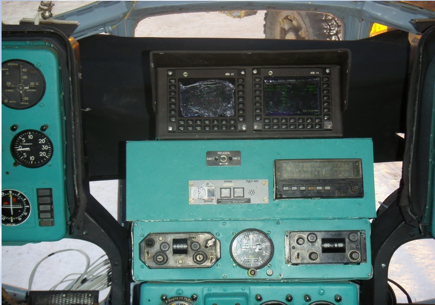
Figure 7. Accommodation of two complete sets of aviation system of navigation «BMS-indicator» in a cabin of crew of helicopter Mi-8AmT
