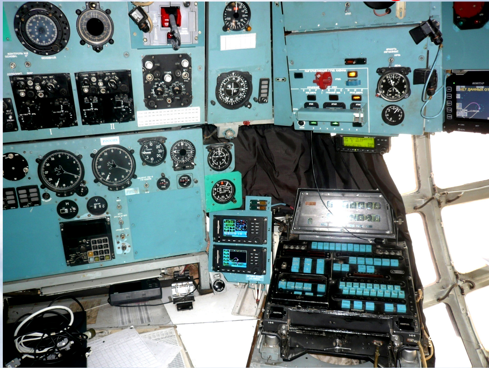
Figure 4. Accommodation of two complete sets by aviation system of navigation SN-4312 in a cabin of the navigator of plane Il-76TD
