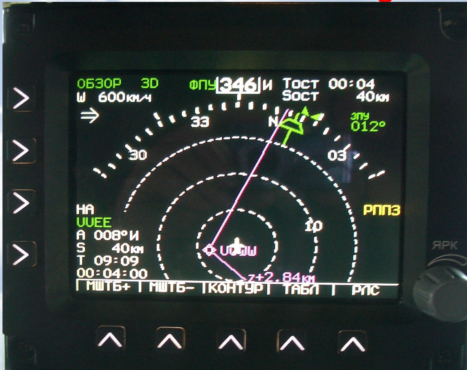
Figure 5. An example of indication of the navigating information acting from SN-4312 on MFI TDS-56D
