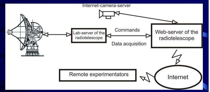
Created remote access system allows carrying out experiments by individual scenarios via global network.
