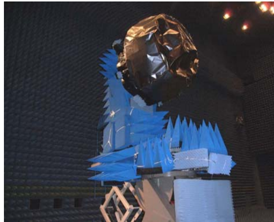
L-band Antenna Pattern Test Proto-Flight Model (July 2008)
