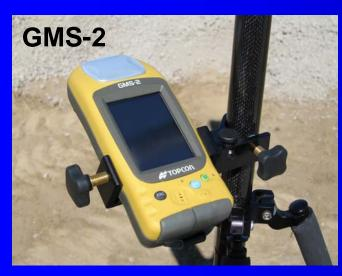
GMS-2: L1 GPS/GLONASS receiver for GIS with camera and compass.
