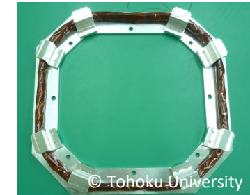
Magnetic Torquers (Electrical Coil)
