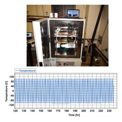
Confirm that the hardware can survive repeated cycles of hot and cold temperature
