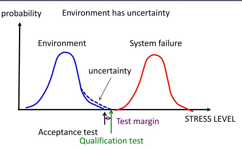
Test at the level higher than the predicted maximum to show that the system is OK even if something unpredicted happen
