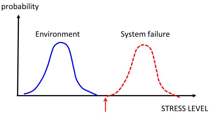
We don't know the lower limit of the system failure
