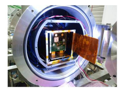
Confirm that the hardware can function at the minimum and maximum temperatures in orbit
