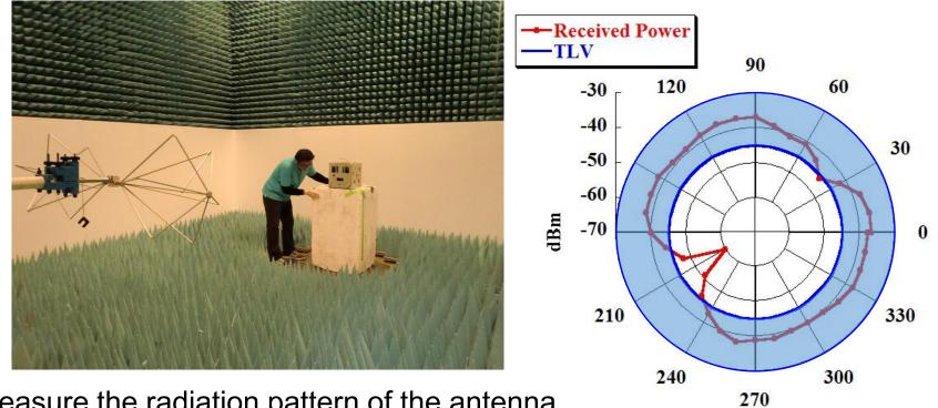
Measure the radiation pattern of the antenna
