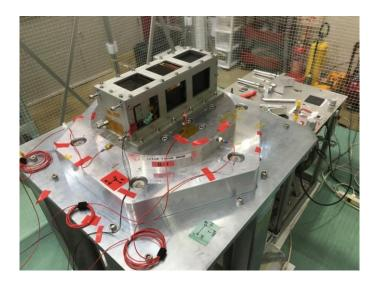
Confirm that the hardware can survive mechanical shock caused by pyro-devices onboard a rocket
