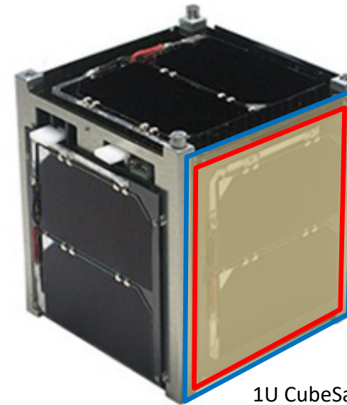
Payload Section Bus System Section
