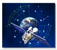
Developer NPO PM Producer PO "Polyot" Total launched 77 SV Ordered 5 SV In orbit 8 SV Clock 5·10<sup>-13</sup> Life-time 4.5 yrs
