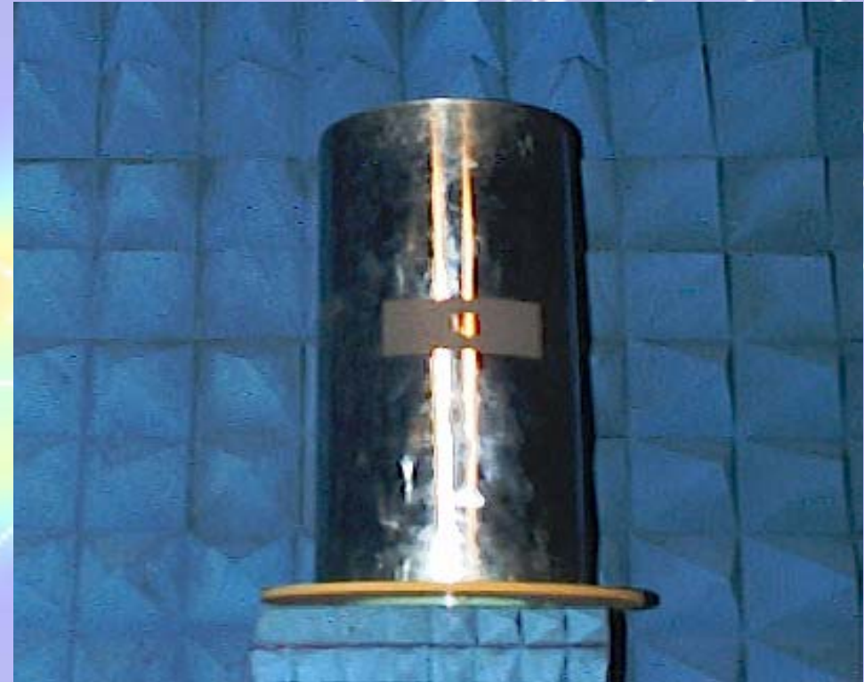
Set up for measurement of the radiation pattern.
