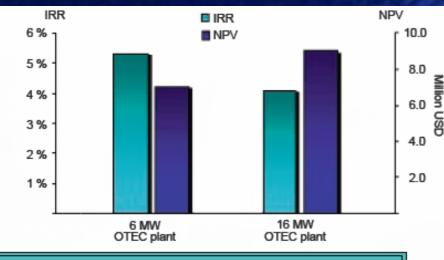
Calculated Net Present Value (NPV) and Internal Rate of Return (IRR) for the reference 6 MW and 16 MW OTEC plants.
