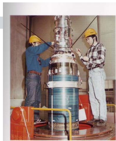
Check-out of a sounding rocket
