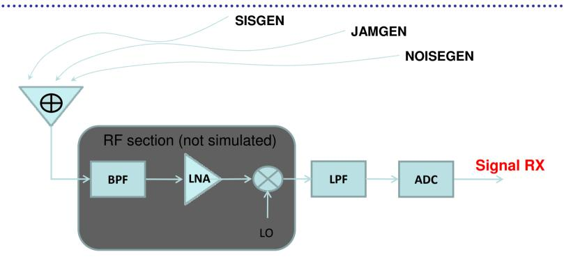
The signal generator is a software package which simulates the received signal at the output of the frontend analog to digital converter
