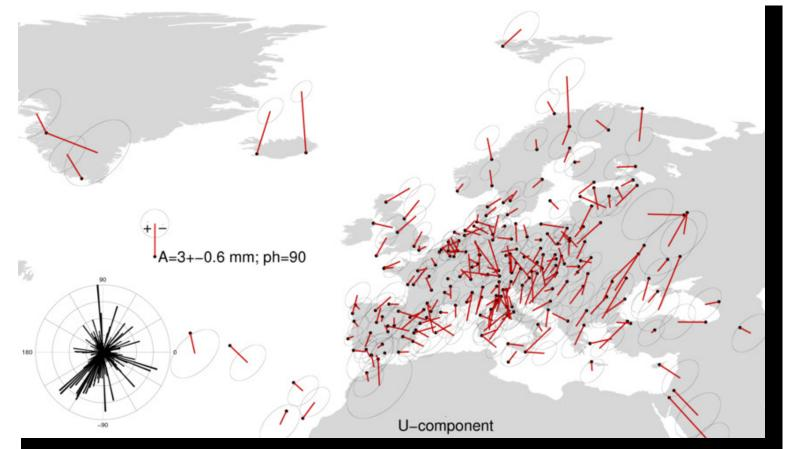
The length of the sticks corresponds to the amplitude and the direction to the phase lag
