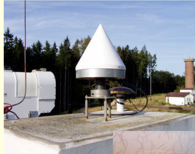
Antenna Topcon CR3-GGD with conical radome
