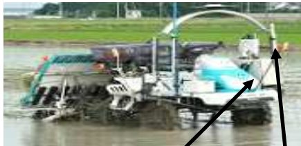
Main Computer GPS Antenna
