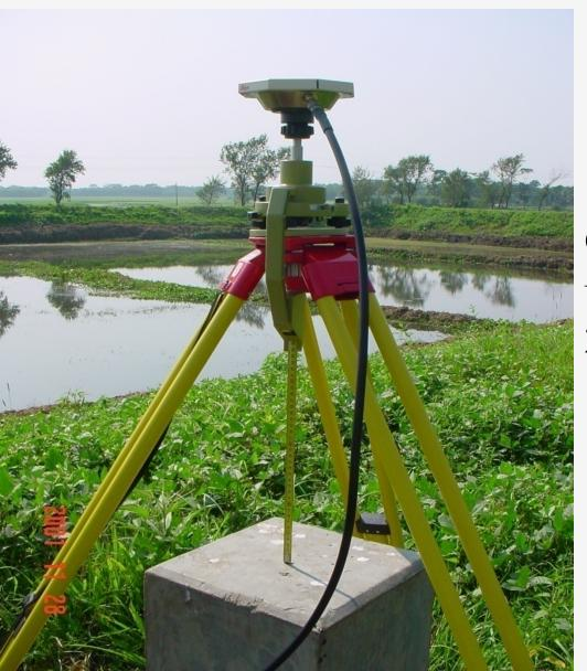
☐ Duel frequency Geodetic Grade GNSS Receiver were used for both 1<sup>st</sup> Order and 2<sup>nd</sup> Order observations
