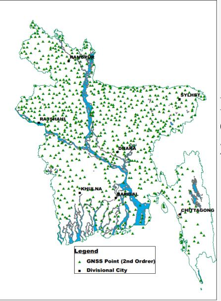
☐ Establishment of Second Order Horizontal Control Points by GNSS survey were started in 2009 and is till continued
