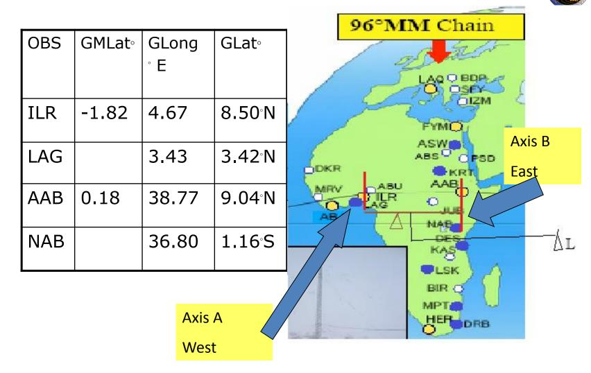
Separation of axes,  $\Delta L = 33.735^{\circ} = 3744.585 \text{ km}$
