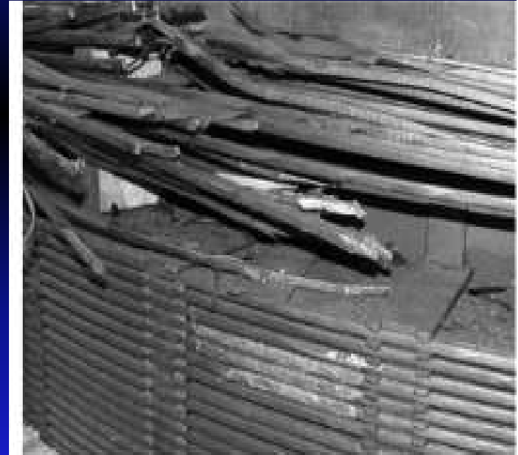
Fig 6: Failure in HV winding of Lethabo #6
