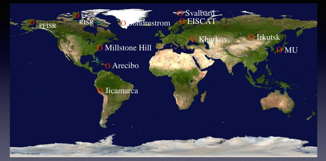
Global Network of High Power Radars Measure Physical Properties of the Space Environment Electron density, electron temperature, ion temperature, plasma velocity, and more...
