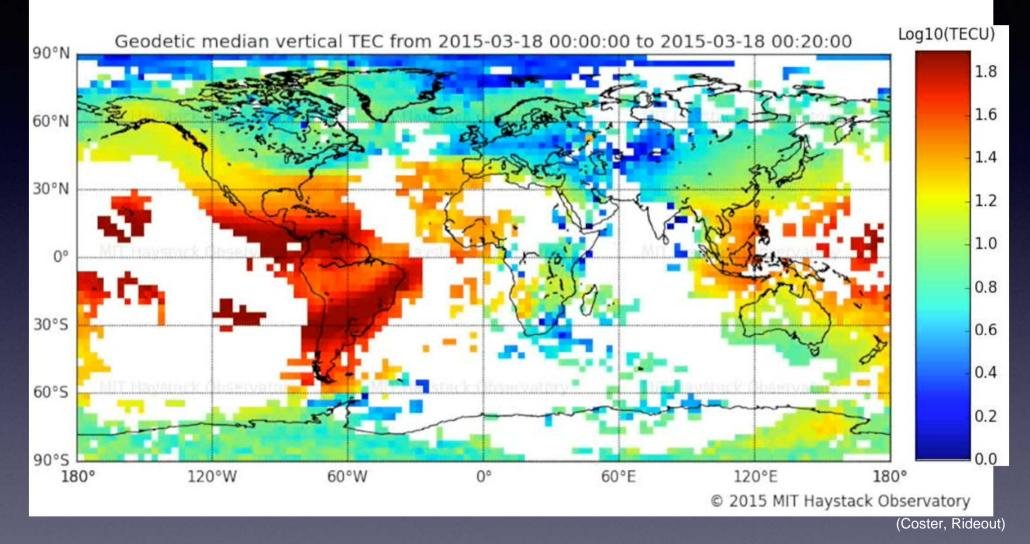
4000+ GNSS geodetic receivers from many sources (e.g. UNAVCO, Scripps Orbit and Permanent Array Center) Processed by MIT Haystack to extract ionospheric delay information Data provides large scale picture of global ionospheric space weather variations Available to space science community through NSF supported Madrigal distributed database
