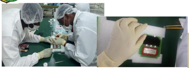
Solar Panel Attachment , three solar panel was broken in the FM development phase
