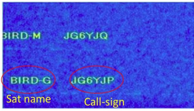
GhanaSat-1 signal reception decoded by Software Define Radio Interface
