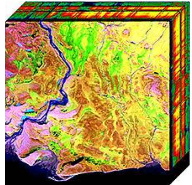
Two-dimensional projection of a hyperspectral cube
