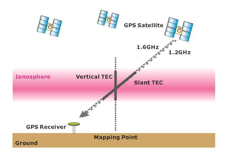
• TEC is the number of electrons in a vertical column that extends from the satellite to the receiver on the Earth.
