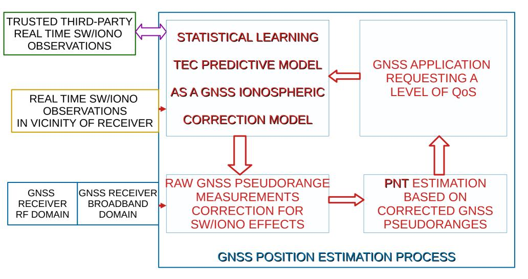
Mitigation of GNSS ionospheric effects using statistical learning-based self-adaptiveness to positioning environment conditions, embedded in GNSS SDR user equipment (R Filjar, *Croatia*) <u>Statistical learning TEC predictive model for GNSS</u> <u>ionospheric delay mitigation – Realisation &</u> <u>demonstration</u>
