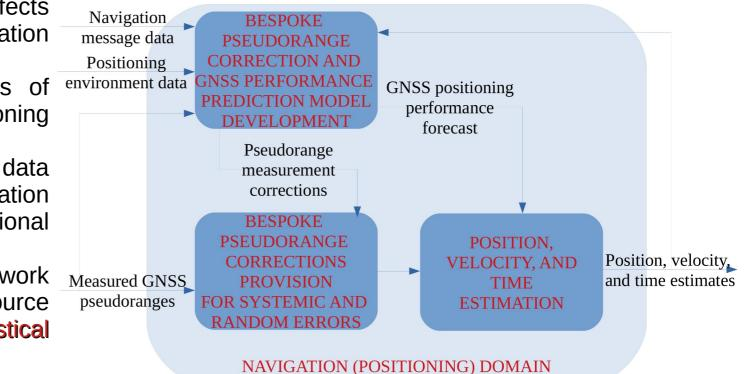
Mitigation of GNSS ionospheric effects using statistical learning-based self-adaptiveness to positioning environment conditions, embedded in GNSS SDR user equipment (R Filjar, Croatia) Demonstration
