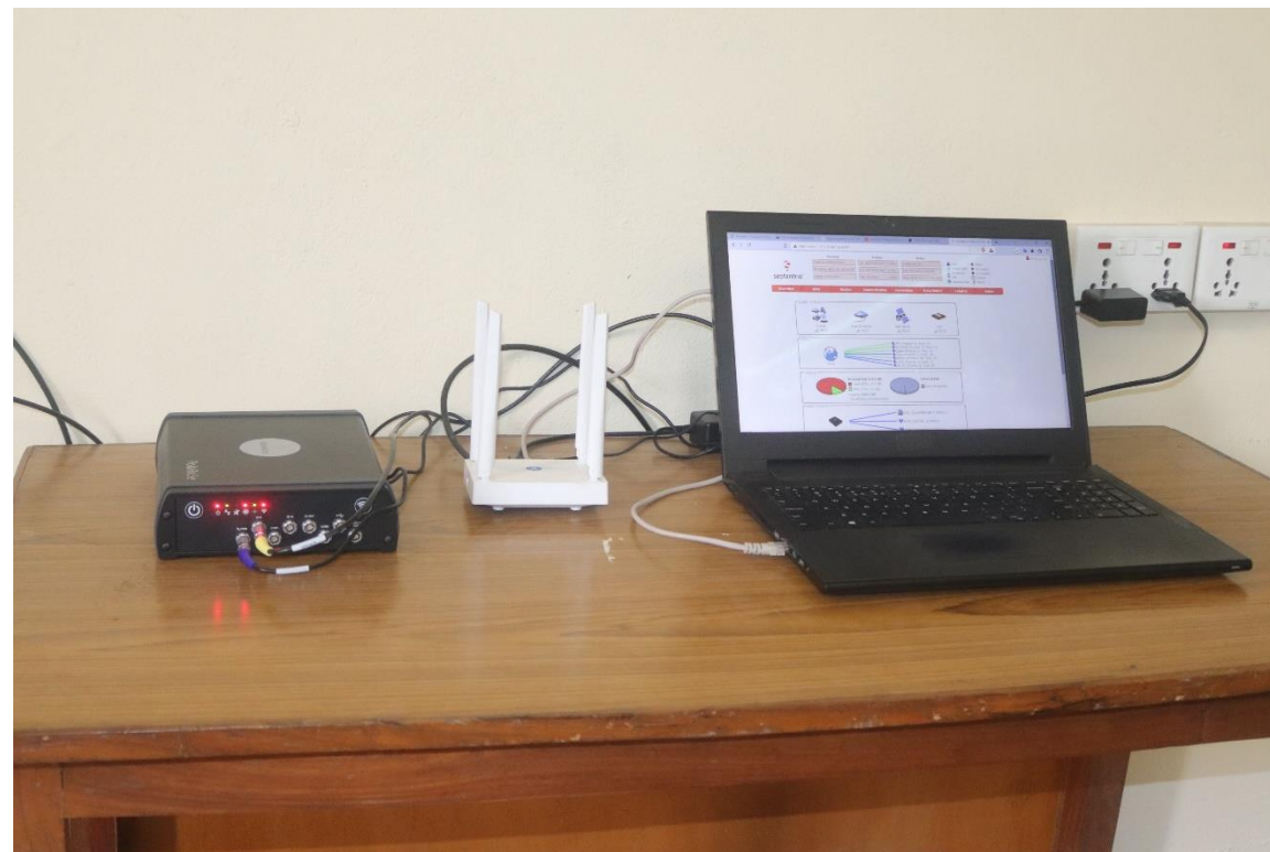
CORS Receiver: PolaRx5 Capable to receive all GNSS signals in all frequencies Data from this receiver is available for R&D
