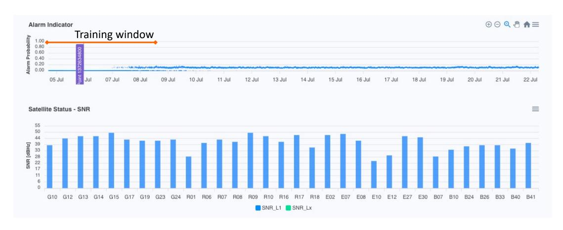
Alarm indicator, and satellite CN0 visibility for each point on the Time Error series.
