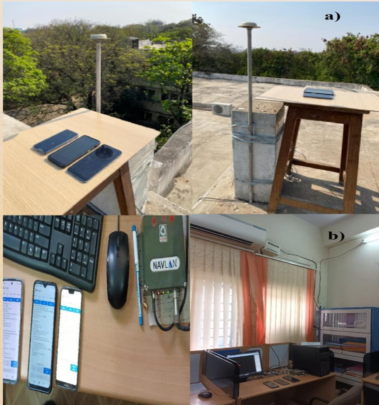
Figure 1. Concurrent GNSS data collection carried out using smartphones at a) outdoor and b) indoor environment conditions.
