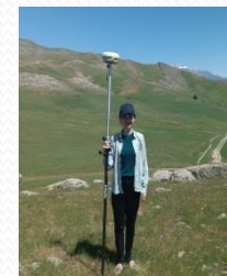
GNSS rover at picket points
