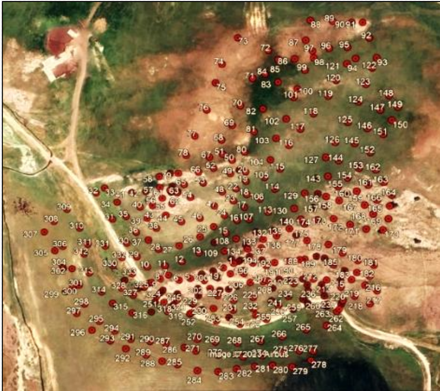
GNSS rover at picket points
