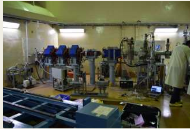
SEL test at Takasaki's reactor
