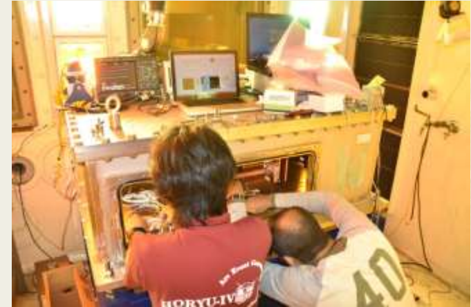
Single Event-latchup test at Kyoto University
