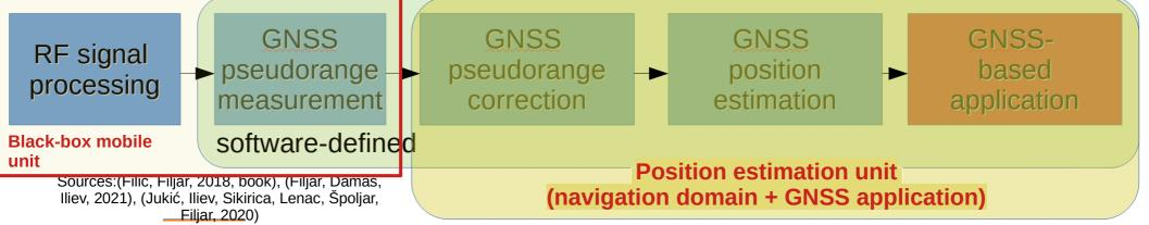
Environment-adaptive GNSS position estimation deployed in distributed GNSS software-defined radio receiver (R Filjar, Croatia)
