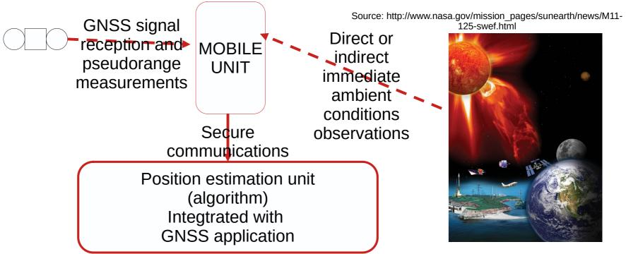
Environment-adaptive GNSS position estimation deployed in distributed GNSS software-defined radio receiver (R Filjar, Croatia)
