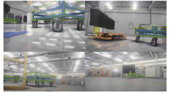
Simulated samples of a dolly (with actual CAD model) used to train object detection and pose estimation neural networks
