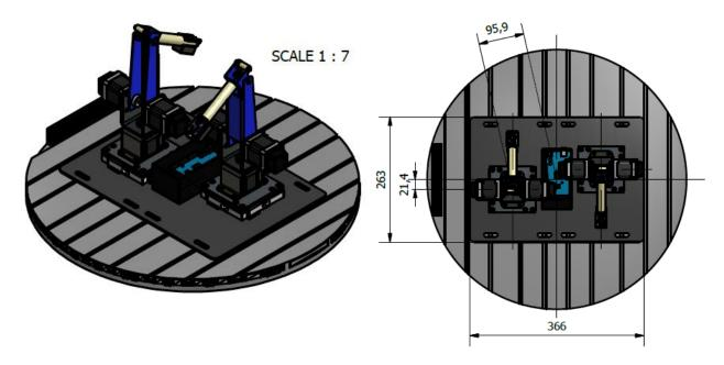
Figure 1: Robotic arm manipulator setup, sketch and dimensions (units in millimeters).
