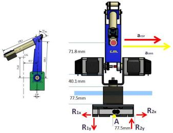
Figure 6: Expected reactions on one arm base.
