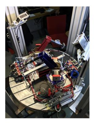
Figure 9. Integrated experiment setup. Image shows the two arms, electronic control, and side cameras integrated in the capsule.
