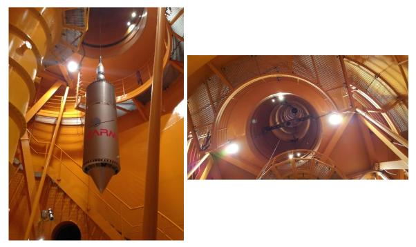
Figure 10. Drop capsule with the experiment prototype integrated in its interior (left). Inner view of the drop path within the ZARM tower (right).
