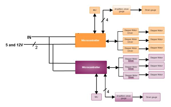
Figure 3: Updated block diagram of the electronic control system for both robotic manipulators used in the experiment.
