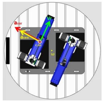
Figure 5. Top view of the structure with induced acceleration vectors on one arm.
