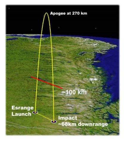
Typical flight trajectory of a microgravity rocket .
