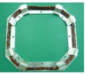
Magnetic Torquers (Electrical Coil)
