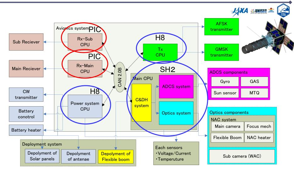
Combination of "High performance but may-be-weak" processor and "Low performance but very robust and space-proven" processor
