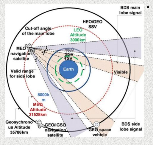
The assumed constellation used for simulation consists of **27 MEO** satellites, 24 out of 27 **MEO** satellites shape up into Walker 24/3/1, and the remaining 3 ones are separately taken as spare satellites in each orbit plane.
