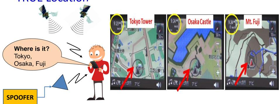
Spoofer transmits signal similar to signals from satellites.
