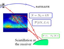
Ionospheric irregularity sensing through multi-scale analysis of radio scintillation on GNSS signals
