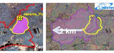
(A) Analysis by Gates Foundation and ESRI using 30 m-resolution DEM (B) Analysis by RESTEC using 5 m-resolution DEM
