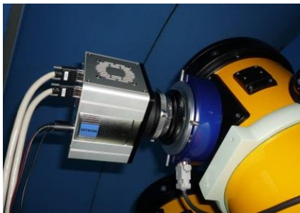
Fig.-2 The CMOS sensor manufactured by Bitran which can detect 10cm LEO objects analyzing the data with FPGA-based image-processing technologies
