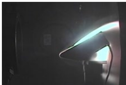
Figure 8 Evaluation tests by arc heating wind tunnel
